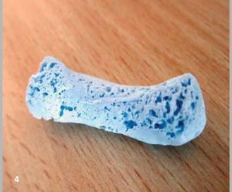
in porous structures which are able to withstand compressive strength of almost 40 MPa (see diagram).
